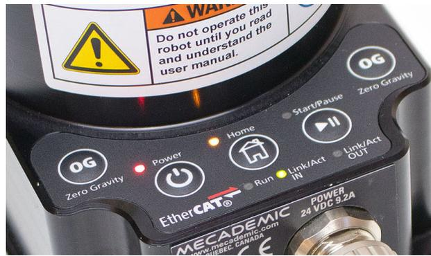
Figure 16: Robot's control panel
